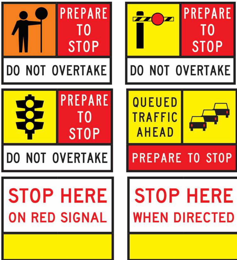
Figure 5.6 – Examples of multi-message sign configuration for traffic control
